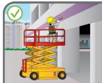
Use suitable working platforms, for example, power-operated elevating working platform or mobile working platform.
